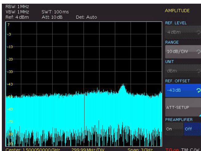
Fig. 6.12: Trace shifting with reference offset
